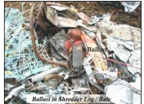
Prohibited: Ballast in shredder log / bale
