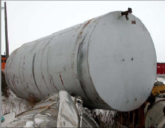
Prohibited: No openings on the tank for inspection
