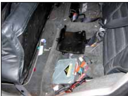
1990 Jeep Cherokee mercury-containing Adaptive Brake Module located under the back seat
