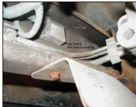
Mercury-containing ABS switch located on the chassis on the underside of Ford Explorer
