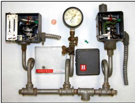
Prohibited: Mercury in pressure and temperature gauges
