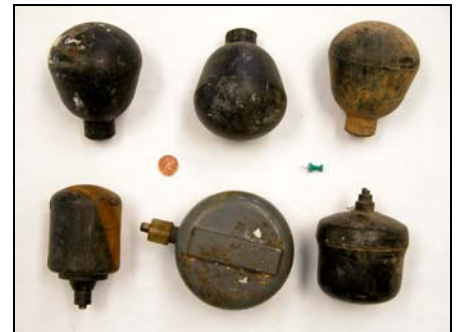
Prohibited: Mercury in level switches
